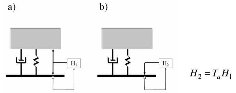
This reformulation helps in the design of compensators and the study of interaction between multiple modules
