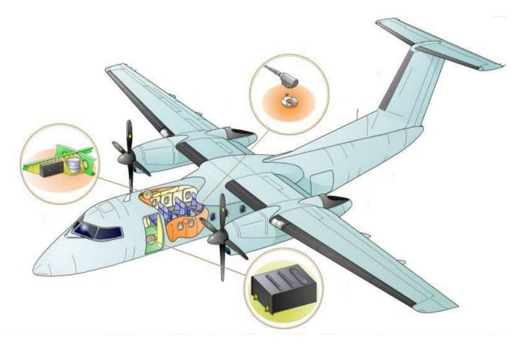
Controller with 46 structural actuators and 72 microphones built by Ultra Electronics and now fitted to over 1,000 aircraft
