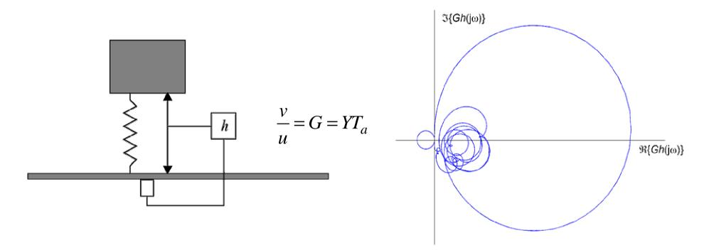
The plate resonances generate loops on the right, corresponding to negative feedback and creating attenuation. The actuator resonance causes a loop on the left, corresponding to positive feedback, causing enhancement and threatening stability
